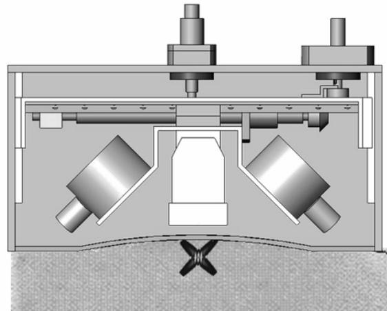
Fig. 1. The scanhead placed upon the surface of the skin. The blue and red cross is a simulated focal zone produced by the dual focused transducers aligned at 90 degrees.
