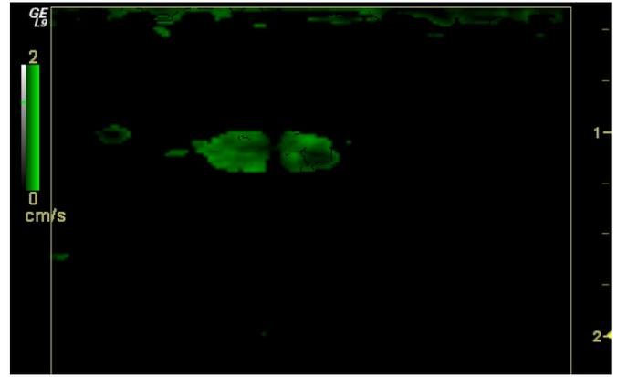
Fig. 4. A variance Doppler image of the stationary acoustic field generated by two focused 1 MHz transducers at a depth of 7 cm. The units of the labels on the right-hand side are centimeters. Notice that the size of the focal region is less than  $0.5$  cm x  $0.3$  cm. The intensity units are relative.
