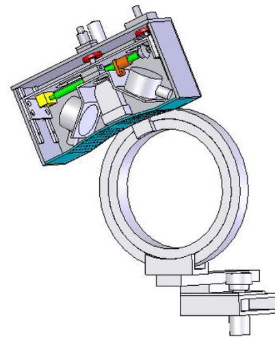
Fig. 2. The five DOF delivery mechanism including the 2 DOF within the scanhead.
