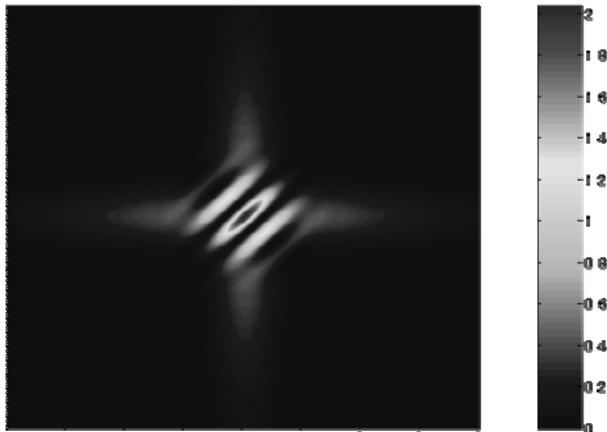
Fig. 3. Computer simulation of the variance of the overlap region of two transducers at 90 degs., calculated for two complete cycles. The diameter of the overlap region is  $3\lambda$ .
